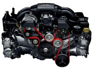
8 Reference the belt diagram above to reinstall the serpentine belt. Reinstall the belt on all of the pulleys but leave the belt off the Revo Alternator pulley.
