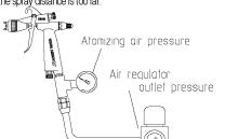
Pulling the trigger of the gun with the pattern adj. Set and fully opened adjust the air regulator in the spray booth to obtain 2.2~4.5 bar (31~64 PSI) at the gun inlet as issued on specifications table ahead. In this way the gun will atomize within 0.7 bar (10 PSI) inside air cap.
