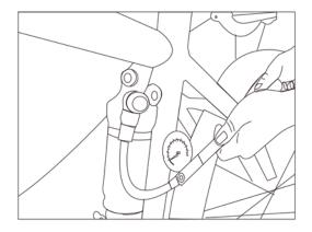
• If pressure needs to be reduced, press the bleeder valve button (red) to release air to your desired pressure.
