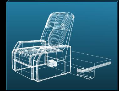
Traditional / Tip-Up seat with BKCS transducer mounted to underside. Wiring from unit is concealed behind seat, and run under seating floor or in wire mold to control room.
