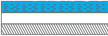
Sanding swirl marks in the substrate show as lines in the top-coat.
