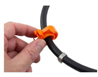
**6.2** Thread the hose clip and retaining clip onto the new hose.
