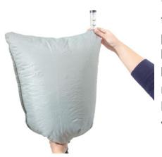
1.4 Place the equipment in the bag and grip the lower part of the bag so that the bag seals around the breathing hose. Grip the flow meter with the other hand and hold it so that the tube points vertically up from the bag.
