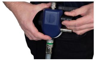
**2.6** Use the regulator knob to set the air flow rate to suit your current work intensity.
