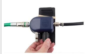
**1.3** Turn the control valve knob anticlockwise as far as it will go in order to throttle the air flow rate to a minimum.
