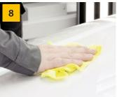
Use Mirka soft micro fibre cloth for final cleaning.
