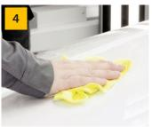
Wipe clean and check the surface. Repeat step 3 if needed. Use Mirka soft micro fibre cloth.
