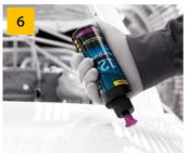
Apply a small amount of **polish** on the polishing pad or directly to the defected surface area.
