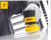
Polish by gently pressing. Use at moderate speed. Wipe clean and check the surface. Repeat if necessary.
