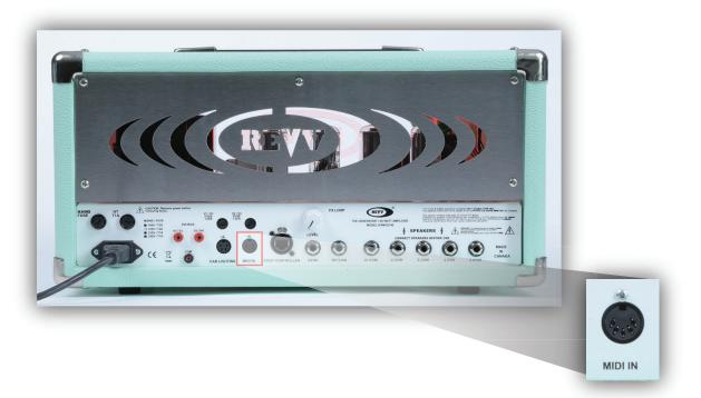
Versatile & optional MIDI control helps Revv amps seamlessly integrate into any rig. The amplifier will store up to 128 programs for program change commands as well as accept Continuous Controller (CC) commands to control functions directly. The amplifier also features OMNI mode to allow control options on 16 channels, & phantom power to power controlling devices.
