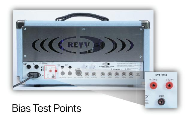
This amplifier is designed to allow the user to set the bias of the power tubes without removing the chassis from the head shell.
