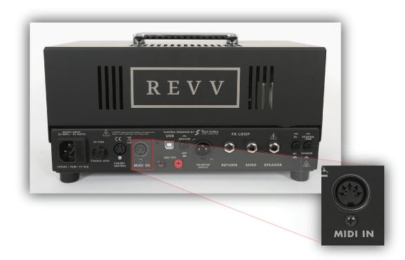
The D20 amplifier is equipped with MIDI for control of the embedded Two notes Torpedo.
