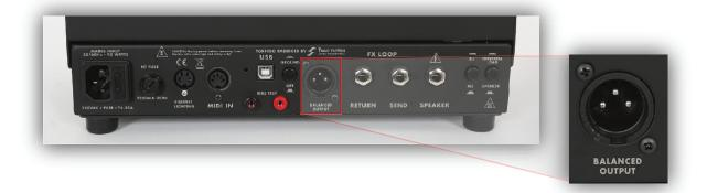
The **balanced out XLR** connector on the rear of the amplifier is a direct output from the embedded **Two notes Torpedo** and not direct from the tube amplifier output itself. The purpose of this output is to be used with audio interfaces to exclude the use of an actual speaker cabinet, using virtual cabinets instead.
