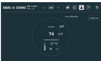
The user can plug any standard BNC pH probe into the unit and measure the pH in the samples at will
