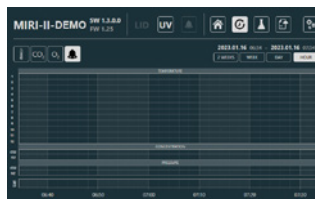
Conditions that put the MIRI® II-12 into alarm state are recorded. It is possible for the software to send email alerts as well.
