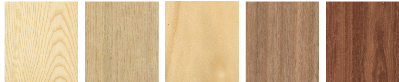
European Ash C European Oak C ¼ Hoop Pine R Ironbark ¼ Jarrah C
