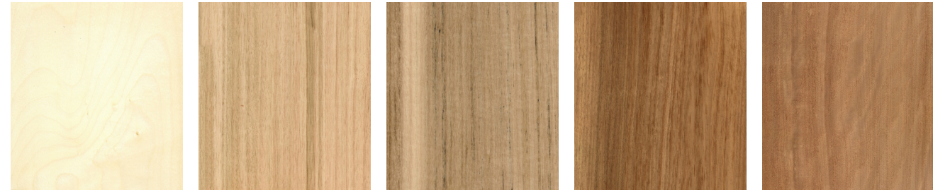
Birch R Blackbutt C ¼ Blackbutt NFG N Blackwood C Brushbox ¼
