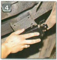
anti-roll bar mounting brackets, Extreme can supply new brackets for fitting to the bare chassis. The chassis bracket set seen here is for a 90/D1/RR Classic (as an illustration). The 110 rear is the only one with the four bolt fixing.
