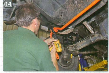
be passing and got roped in to help hold up the heavy rear anti-roll bar while the polyurethane bushes were slid into their correct locations. Ian attempted to fit all the mounting bolts but hit a snag.
