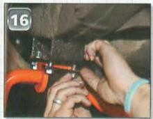
welded-on mounting bracket with two different sizes of hole: 10 mm and 8 mm. Of course, you don't notice it until you start to fit the bolts! Ian carefully drilled out the 8mm holes...
