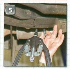
before inserting the rivnuts to provide captive nuts in the chassis. New rivnuts are supplied with the kit and Extreme also sell an excellent riv-nut tool to set the M10 riv-nuts into the chassis. (It also does other size riv-nuts for light guards and similar accessories.) It retails at \$37.45 plus VAT.
