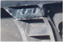
13) At rear, slider butts up to blank-ended outriggers. This one's under rear door.
