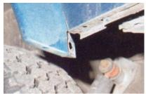
3) Remove the nut and bolt at each end of the sill (they lock the plastic arch to it.)
