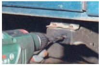
15) Remove rock slider and drill the four 10mm holes in the two outriggers.
