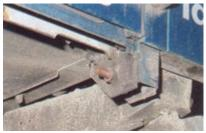
7) When the sill's off, remove this large bolt, smear it with copper grease and refit.
