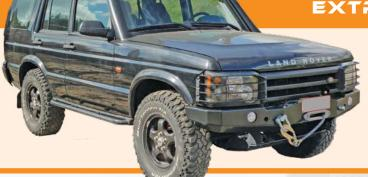
This winch bumper offers great protection. Spoiler and front skirt will require removal. Superb approach angle and body protection. The bumper has provision for 2 swivel recovery eyes to help prevent winch cables twisting. 2 built-in Hi-Lift Jacking points. Choice of driving or fog lights (included). Zinc primed & powder coated.
