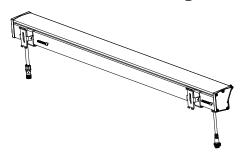
• Take out the metal hoop in the accessory bag, pass through the beam of the stadium fence, and cross the corresponding card position of the lamp mounting base, and tighten the fastening screws.
