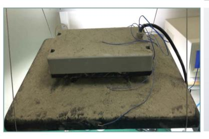
In order to simulate that under dusty working environment for 5 years time, the whole fixture was fulfilled with dust. Then the temperature of LED and Driver Tc increase 2 degrees only.
