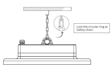
•Check that the fixing is correct before connecting the wiring. If the luminaire is held securely, proceed with the connection of the luminaire to the power supply.
