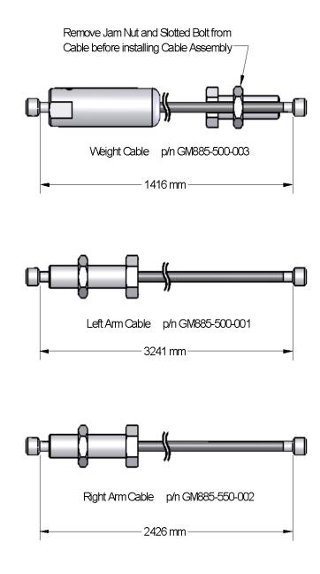
Cable lengths are in millimeters and for reference only. Cable lengths could change at any time without notice.
