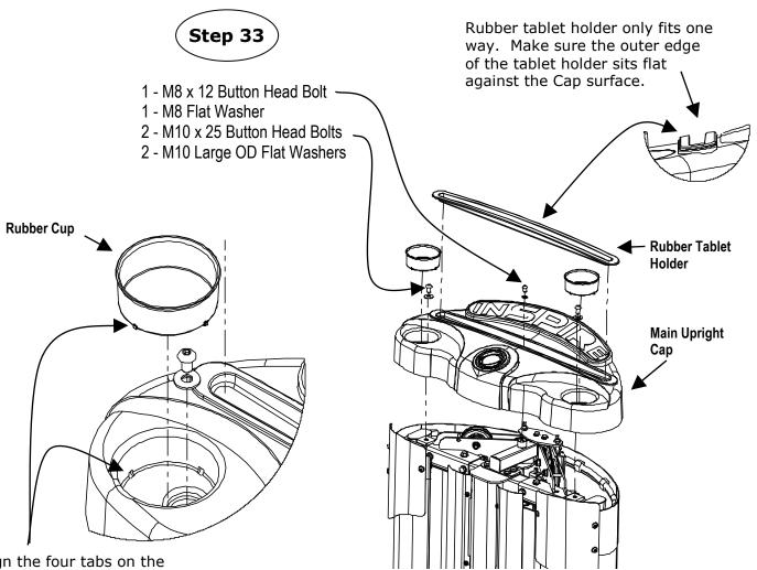
Align the four tabs on the bottom of the rubber cup with the notches in the bottom of the pocket.
