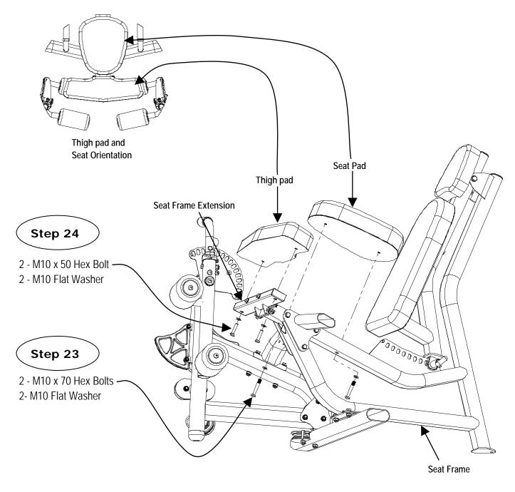
Step 23: Attach Seat pad to Seat Frame using:
