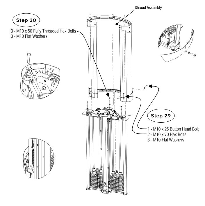
Step 29: Attach the Lower Metal Shroud to the Upright 1 and Main Frame using:
