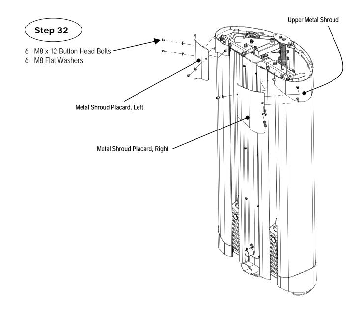
Step 32: Attach the Metal Shroud Placard to the Upper Metal Shroud using:
