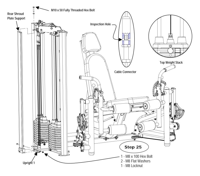
Step 25: Attach the Rear Shroud Plate Support to Upright 1 using:
