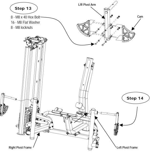
Step 13: Attach Cams to Both Left and Right Pivot Arm using:
