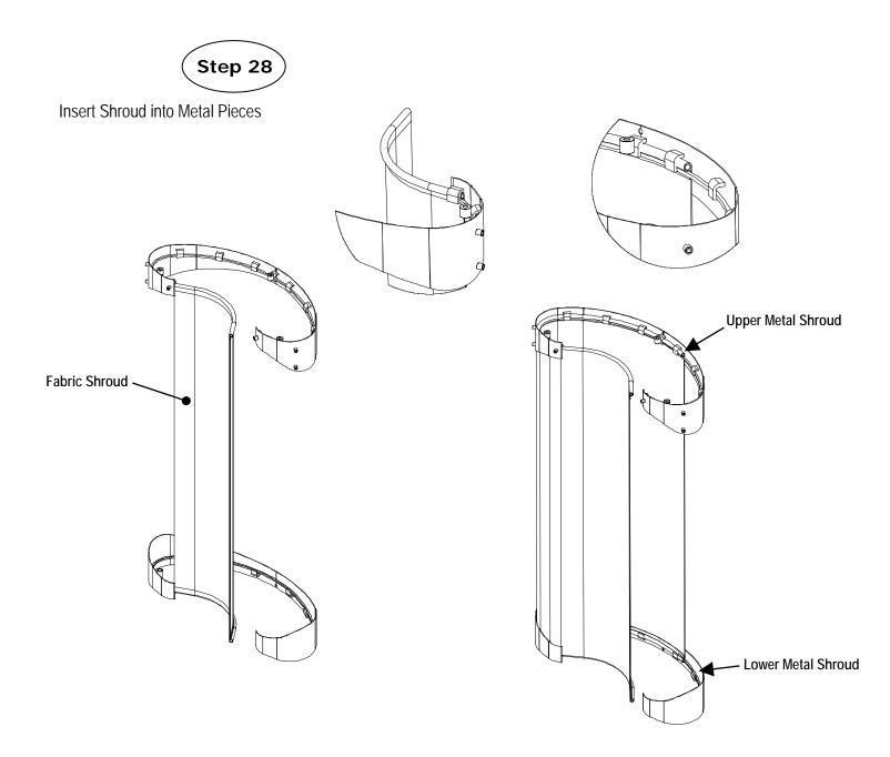
Step 28: To install Fabric Shroud, start from one end of the Lower Metal Shroud and insert the Fabric Shroud inwards as shown. Make sure to have the same orientation as shown or else the fabric shroud will be installed backwards. Continue to pull the Fabric Shroud along the inside of the Lower Metal Shroud until it approaches the other end.
