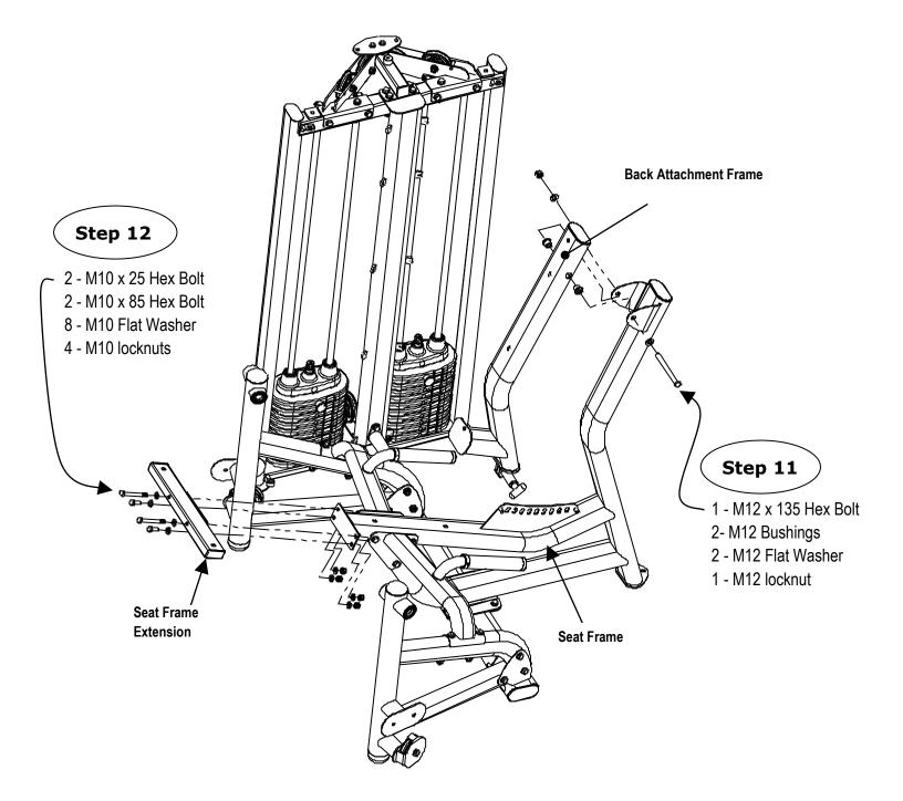
Step 11: Attach Back Adjustment Frame to Seat Frame using:
