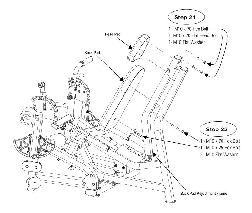
Step 21: Attach Head pad to Back pad Adjustment Frame using:
