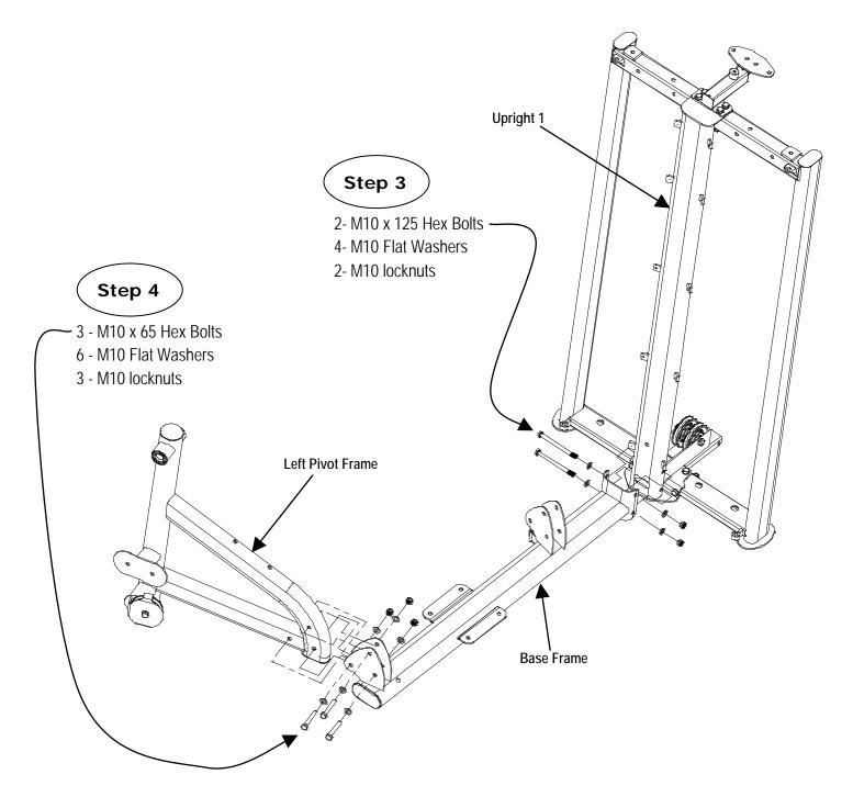
Step 3: Attach the Base Frame to Upright 1 using:
