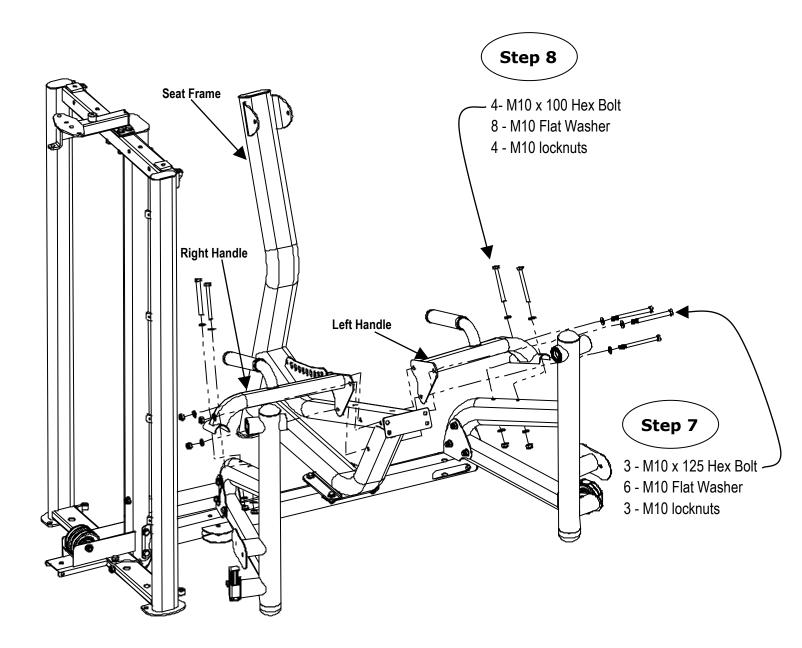
Step 7: Attach Left Handle and Right Handle to Seat Frame using:
