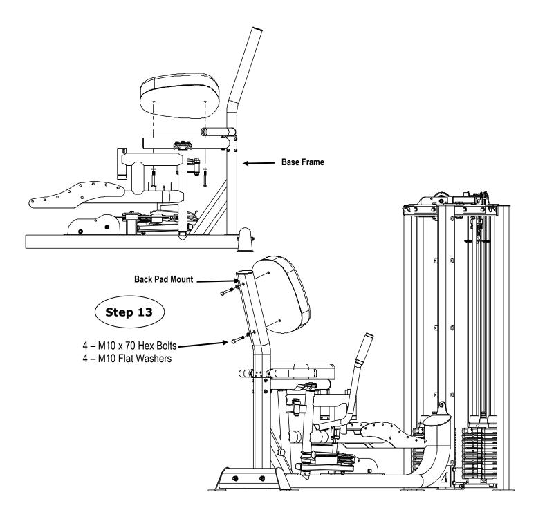
Step 13: Attach the Seat Pad to the Base Frame and Back Pad to Back Pad Mount using:
