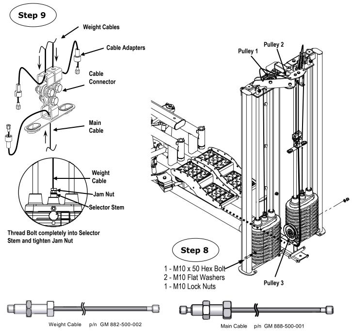
Step 8: Route the Main Cable through the upright and then install Pulley 3 using:
