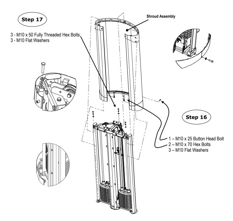
Step 16: Attach the Lower Metal Shroud to the Upright 1 and Main Frame using:
