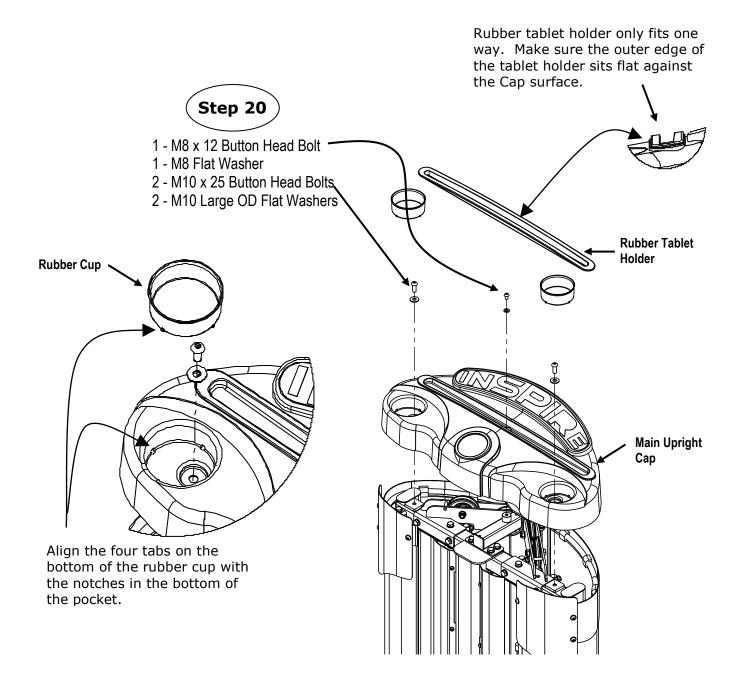
Step 20: Attach the Main Upright Cap to the Main Frame using:
