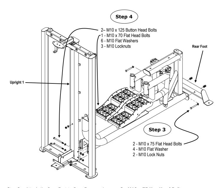
Step 3: Attach the Rear Foot to Base Frame using: 2 - M10 x 75
