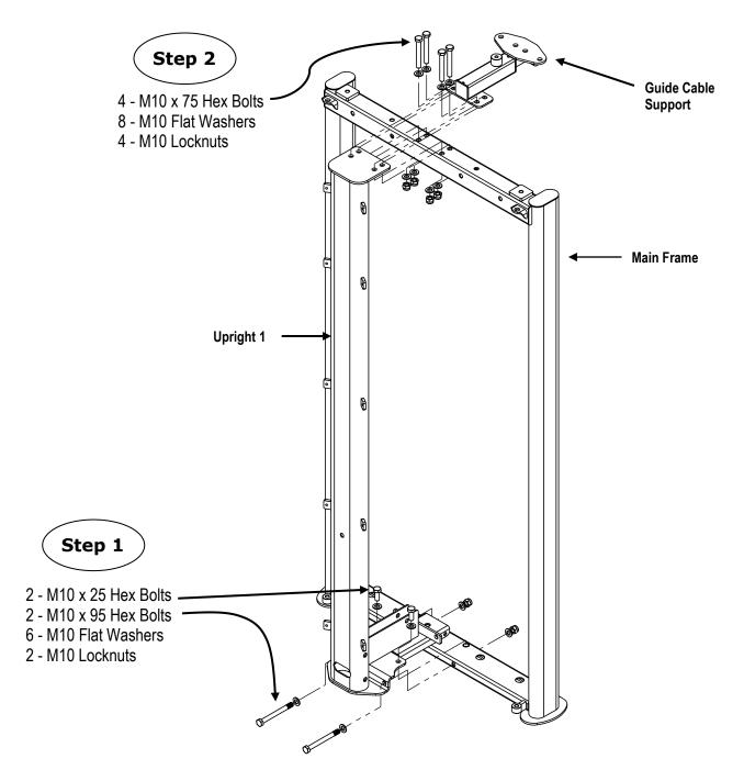
Step 1: Attach Upright 1 to the Main Frame using:
