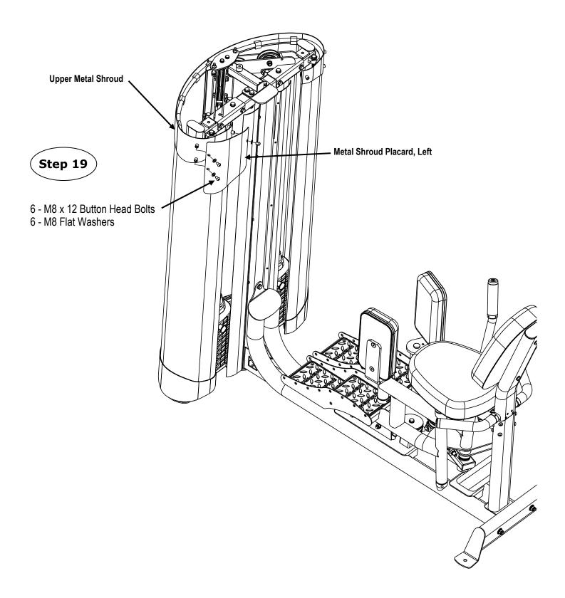
Step 19: Attach the Left and Right Metal Shroud Placard to the
