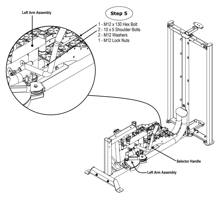
Step 5: Attach the Selector Handle to Left Arm Assembly using: 1 - M12 x 130 Hex Head Bolts
