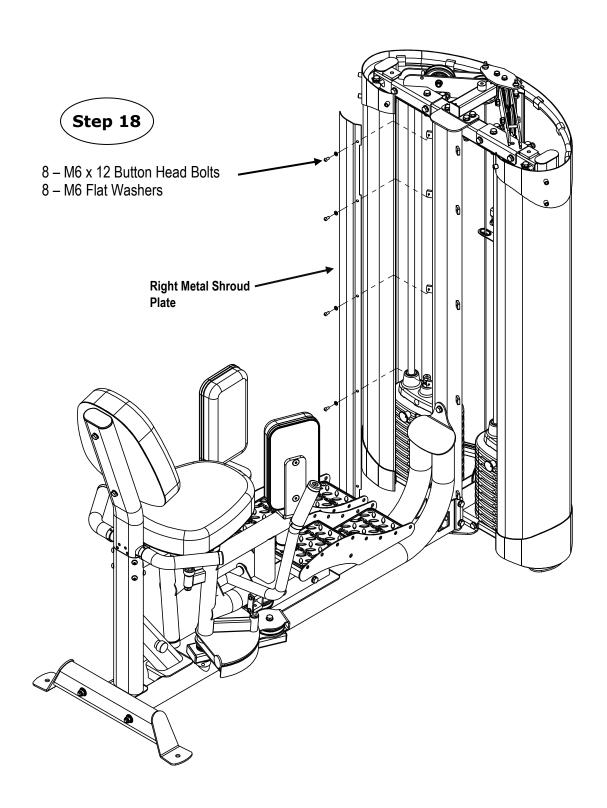
Step 18: Attach Right and Left Metal Shroud Plates to Upright 1 using:
