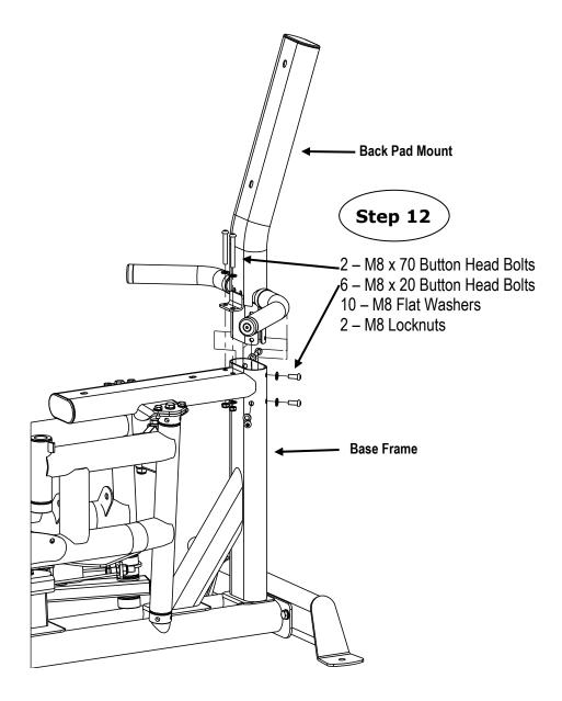
Step 12: Attach the Back Pad Mount to the Base Frame using:
