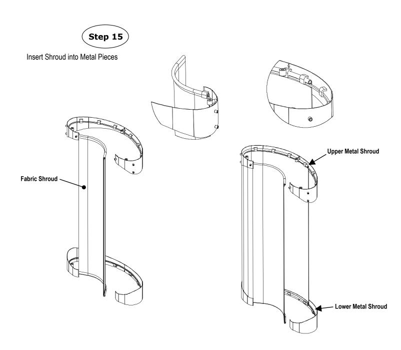
Step 15: To install Fabric Shroud, start from one end of the Lower Metal Shroud and insert the Fabric Shroud inwards as shown. Make sure to have the same orientation as shown or else the fabric shroud will be installed backwards. Continue to pull the Fabric Shroud along the inside of the Lower Metal Shroud until it approaches the other end.
