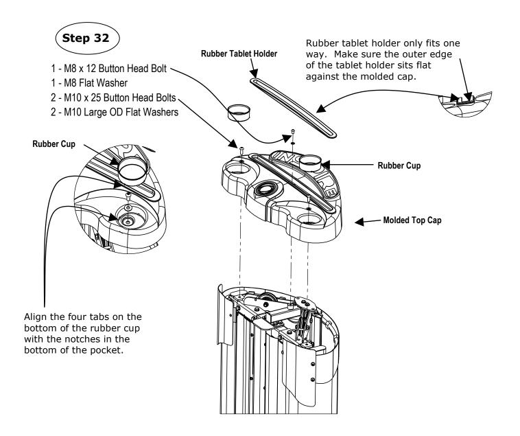
Step 32: Attach the Molded Top Cap to the Main Frame using:
