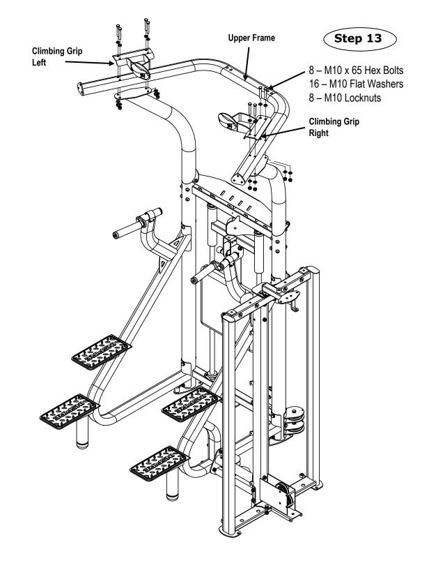
Step 13: Attach the Upper Frame, Climbing Grip Left and Right to the 2 Upper Arms using:
