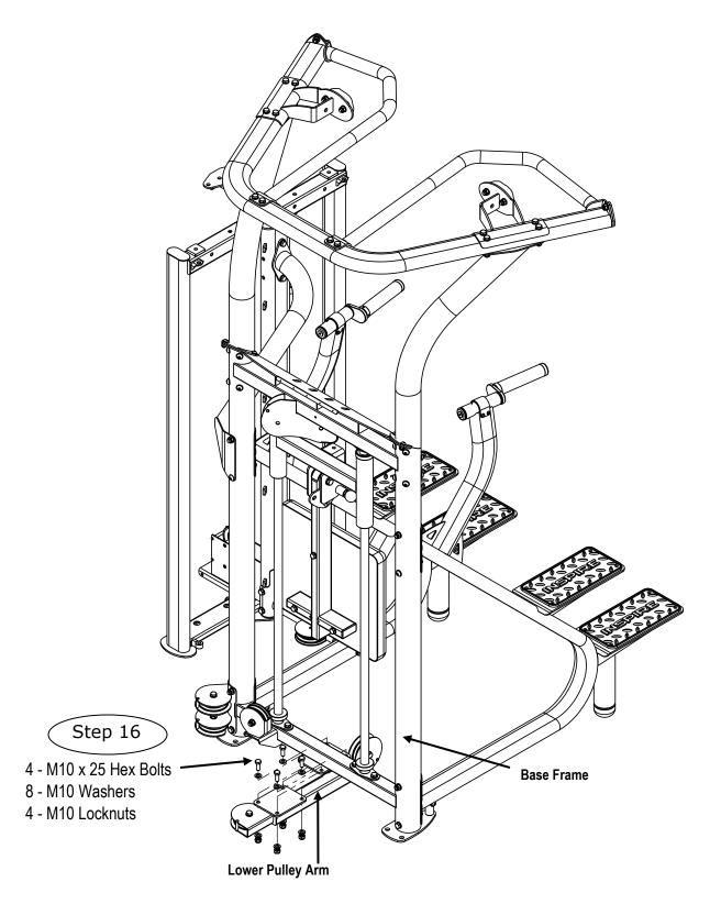
Step 16: Attach the Lower Pulley Arm to the bottom of Base Frame using:
