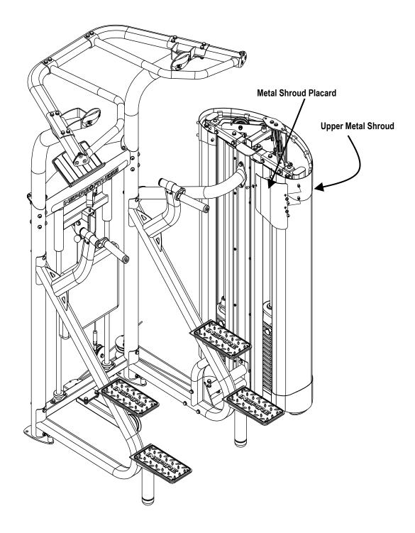
Step 30: Attach the Metal Shroud Placard to the Upper Metal Shroud using:
