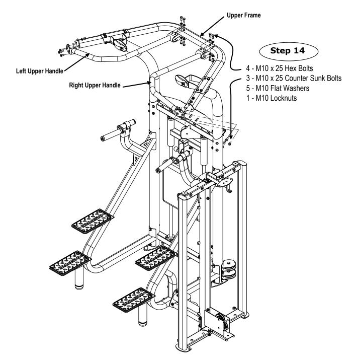
Step 14: Attach the Left Upper Handle to the Upper Frame using:
