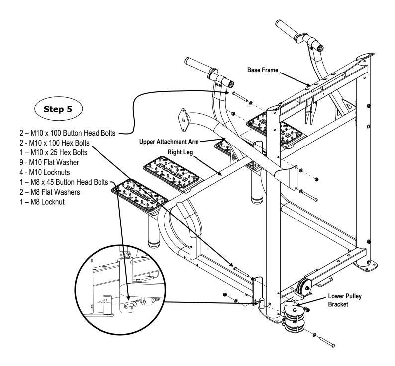
Step 5: Attach the Right Leg, Base Frame, Upper Attachment Arm and Lower Pulley Bracket using:
