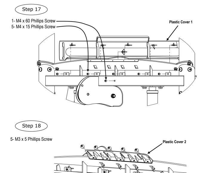
Step 17: Attach Plastic Cover 1 to Base Frame using:
