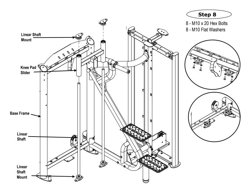
Step 7: Carefully install the Linear Shafts into the Linear Bearings in the Knee Pad Slider. Attach the bottom Linear Shaft Mounts to the Shafts and tighten the set screws. Install the top Linear Shaft Mounts to the Linear Shaft, but do not tighten set screws.
