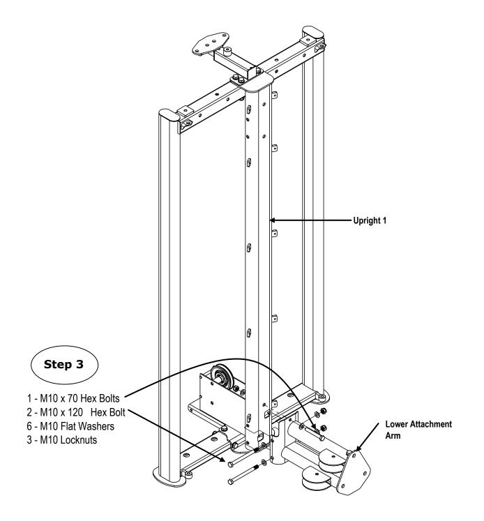
Step 3: Attach the Lower Attachment Arm to Upright 1 using:
