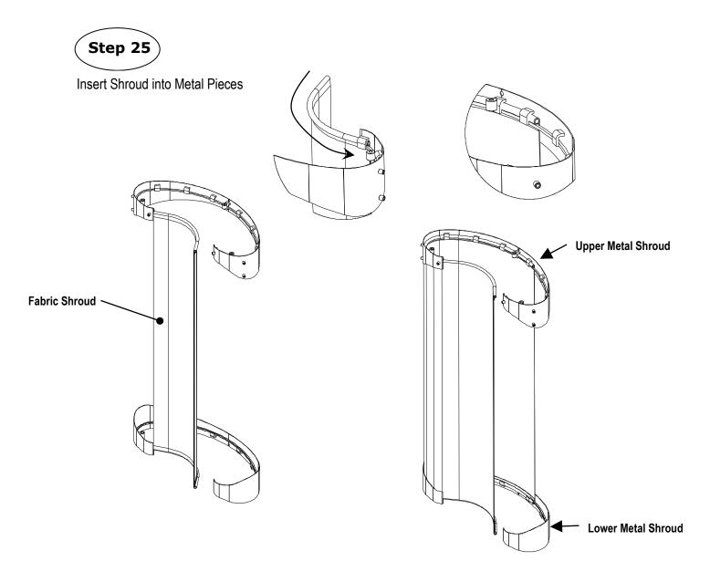
Step 25: To install Fabric Shroud, start from one end of the Lower Metal Shroud and insert the Fabric Shroud inwards as shown. Make sure to have the same orientation as shown or else the fabric shroud will be installed backwards. Continue to pull the Fabric Shroud along the inside of the Lower Metal Shroud until it approaches the other end.
