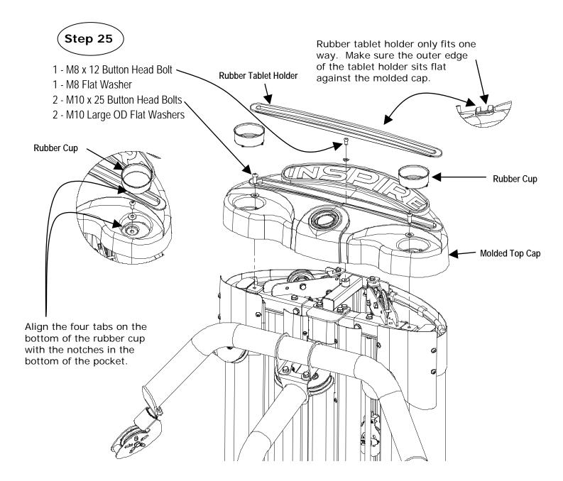
Step 25: Attach the Molded Top Cap to the Main Frame using:
