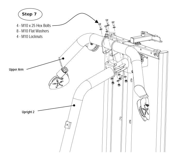
Step 6: Attach the Upper Arm to the Upright 2 using:
