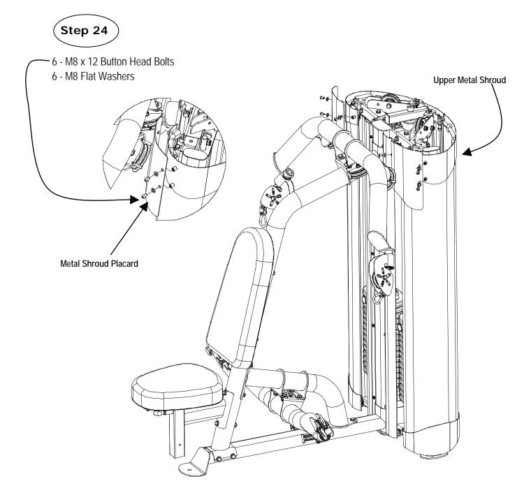
Step 24: Attach the Metal Shroud Placard to the Upper Metal Shroud using:
