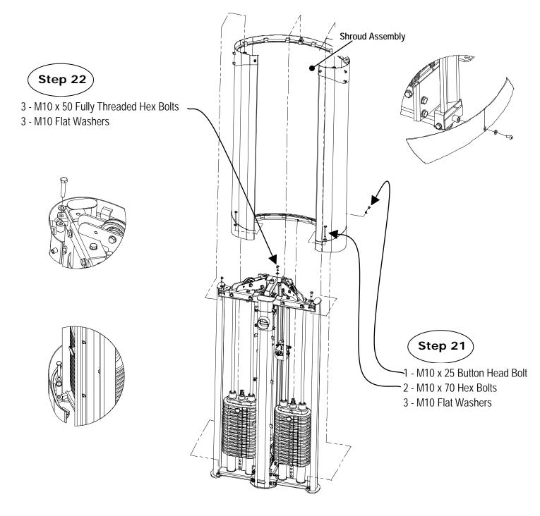
Step 21: Attach the Lower Metal Shroud to the Upright 1 and Main Frame using:
