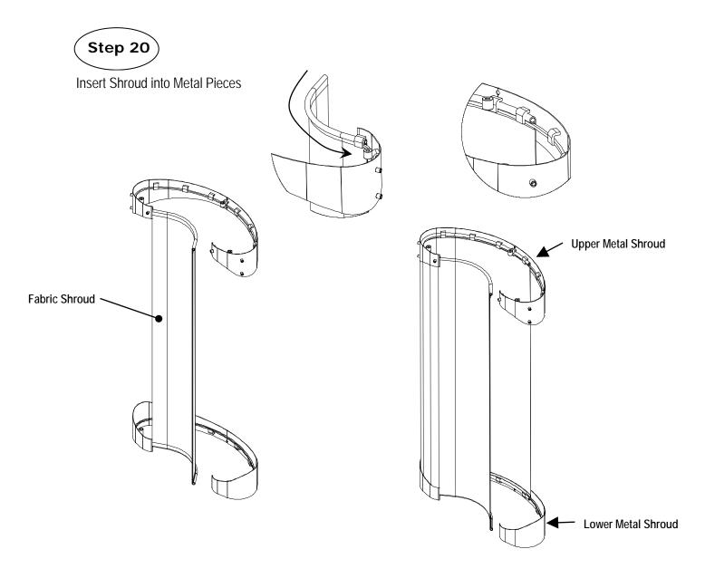
Step 20: To install Fabric Shroud, start from one end of the Lower Metal Shroud and insert the Fabric Shroud inwards as shown. Make sure to have the same orientation as shown or else the fabric shroud will be installed backwards. Continue to pull the Fabric Shroud along the inside of the Lower Metal Shroud until it approaches the other end.
