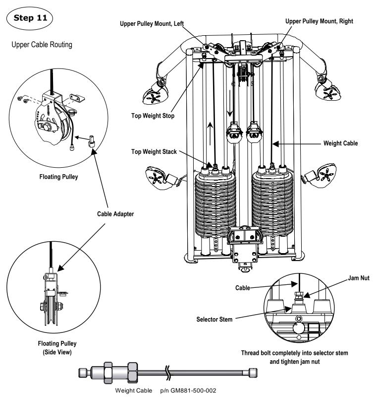
Step 11: Insert the Hex Bolt end of the Weight Cable into the Top Weight Stack. Take the other end of the Weight Cable and guide it straight up through the Top Weight Stop and around both of the pulleys in the Upper Pulley Mount, Left. Attach the Floating Pulley to the cable end as shown. You may need to unscrew the tiny screws in order for the cable adapter to fit.
