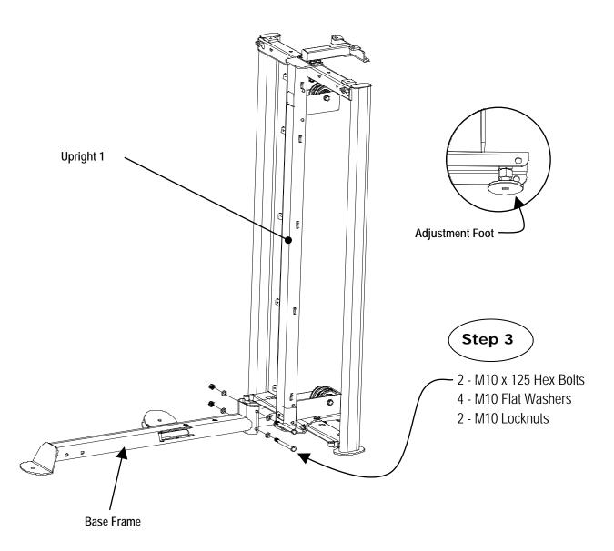
Step 3: Attach the Base Frame to the Upright 1 using:
