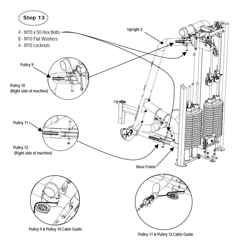
Step 13: When inserting Pulley 9 and Pulley 11, make sure the cables are in front of the pulleys and are in the pulley grooves; not above or below the pulley. Attach the Pulley to the Base Frame using:
