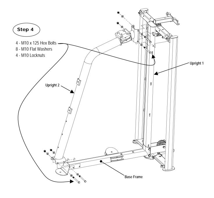
Step 4: Attach the Upright 2 to the Base Frame and Upright 1 using:
