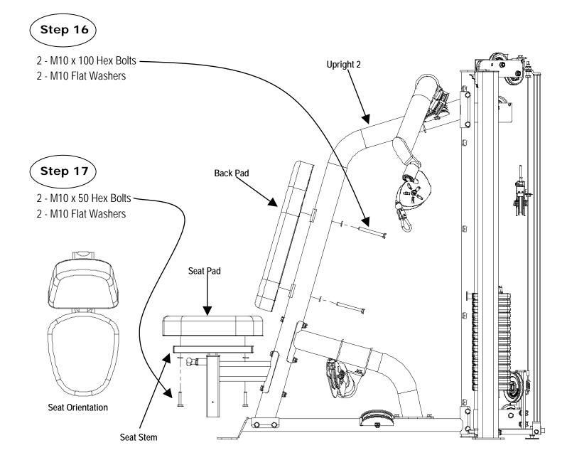
Step 16: Attach the Back Pad to the Upright 2 using:
