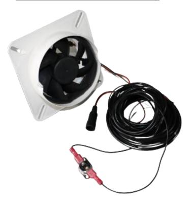
An integrated plastic intake air collar, axial DC air fan, 2x thermostat leads, 30°C thermal switch with connectors and 2.1mm Female DC Power plug. This is the same air intake assembly used in the 1500 Series Solar Air Heater, Get 2, available for individual sale for use in DIY solar air heater projects.
