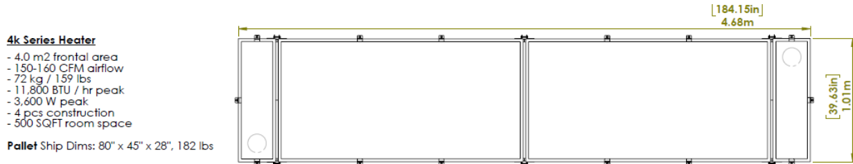
Figure 1: 4000 Series, Gen 1 Heater Specifications and Overall Dimensions
