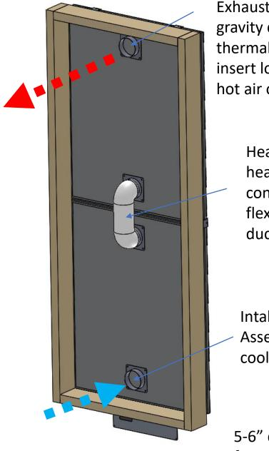
Exhaust collar with gravity damper + thermal switch insert location – hot air out
