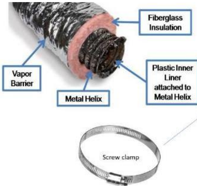
Connect the 4" insulated ducting inside liner to the heater intake and exhaust using screw clamps as shown above
