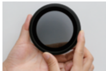
Screw the Circular Polariser for M100 into the holder ring.
