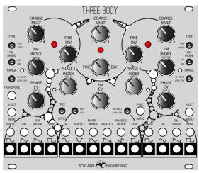
The four small LEDs across the middle are all tied to the output of the index VCA next to it. This way you will see both the intensity and the rate of the modulation.
