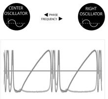
This is also one of the reasons that phase modulation was substituted for exponential frequency modulation in ratio mode, the other is that exponential modulation with ratios does not make a lot of sense (and was difficult to accomplish for various technical reasons related to the architecture of the system).
