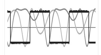
Another method to create a stereo image is to use one output each from the outer oscillators in ratio mode where they are tracking the center oscillator. They will be locked to some frequency ratio but are still free running (not phase locked). This can provide the illusion of a single source but a wide stereo field and can be enhanced by using cross modulation between the two. The more modulation is used the more pitch differences are perceived as timbre changes instead.
