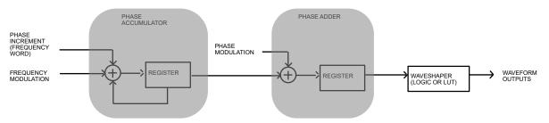
A traditional digital oscillator (direct digital synthesis or DDS) is accomplished with an accumulator. The accumulator can also be thought of as a counter, where each clock tick some amount is added to the counter along with the previous value of the counter. This can be visualized as a stepped sawtooth waveform.
