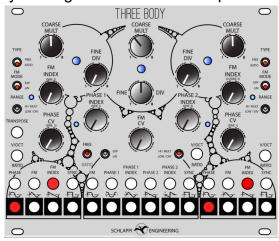
Make sure all modulation controls are fully counter clockwise.
