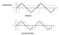
The tracking measurement is taken the rising edge of a comparator set around a volt and ends at the next rising edge, and is averaged over 8 measurements. This means pulse width is not important but it may take moment to exactly match a quickly changing signal.
