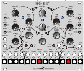
If the division (the FINE DIV knob) of the right oscillator is set to one (fully counter clockwise) then turning the multiplication (COARSE MULT) will travel up and down the harmonic series.
