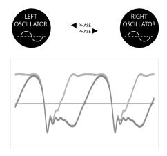
Cross modulating two oscillators with frequency modulation (either with frequency modulation both ways or phase one way and frequency the other) will cause pitch instabilities and rather unpredictable behavior. It may also cause one oscillator to lock on to another or to cease oscillating independently. It is recommended not to do this when you are attempting a melodic patch or looking for anything other than unpredictability and chaos.
