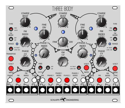
All input controls should be fully counter clockwise (FM INDEX, PHASE CV, PHASE INDEX, FM CV)
