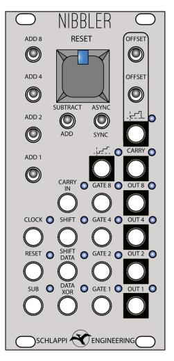
The interface is designed to to be playable, with switches for the binary counting as well as two mode switches and two phase offset switches (so the second stepped analog output can be offset in phase from the first). There is also a large Cherry MX Brown keyboard switch for resetting the register to zero.
