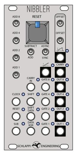
The interface is designed to to be playable, with switches for the binary counting as well as two mode switches and two phase offset switches (so the second stepped analog output can be offset in phase from the first). There is also a large Cherry MX Brown keyboard switch for resetting the register to zero.
