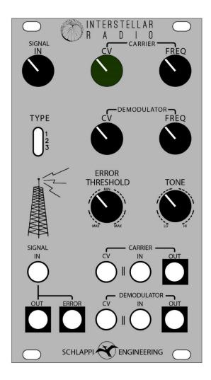
The Interstellar Radio is a faulty transmission line providing several varieties of destructive effects as well as acting as a non-volts/octave complex oscillator when no input is provided.
