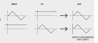
When used as a ring modulator with the cycling slew you may want to use the negative switch on the bias to offset the unipolar signal into a bipolar signal.
