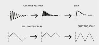
The rectify input can also be used as part of a frequency doubler (with triangle input) or waveshaper (with most other waveforms.
