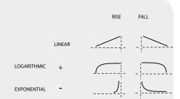
This is done by normalizing the output (feedback) as voltage control. If the output is high it will provide more control voltage and this can (for example) cause the fall shape to start fast then go slower as it drops. Or if the output is low it will start slow then speed up providing an exponential curve. The opposite will occur if the inverting switches are used.
