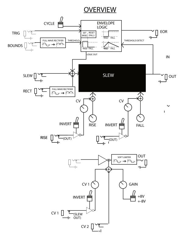
(parentheses indicate connections normalled to unconnected inputs)
