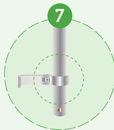
Place the Collar Clamp back onto the handle stem above the holding button
