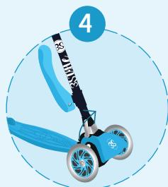
This will release the lock mechanism from its holding recess, allowing you to pull up the handles
