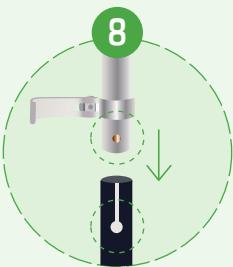
Place the handle stem back into the top of the main stem, taking care to line up the holding button with the holes on the side of the stem
