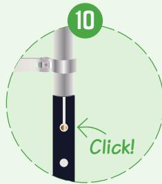
The button should spring out into a locked position at the first hole. (Don't be afraid to give it a wiggle to get it seated)
