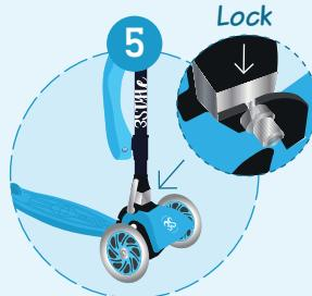
Lift scooter handles to up position. Scooter lock mechanism will fall into its locked position
