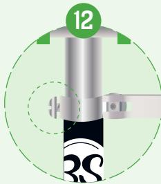
Place the screw back in and tighten to secure the Collar Clamp once more. You are now ready to go!
