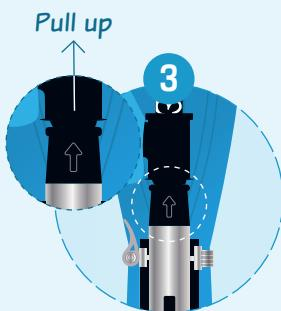
Pull up on scooter release pump & hold in open position
