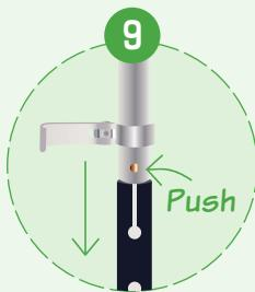
Push the Holding button in and push the handle stem down into the main stem
