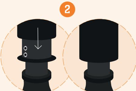
Position the seat so that its guiding notch allows it to fall correctly into position on top of the holding ring
