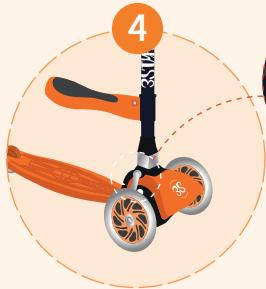
Close the scooter lock mechanism
