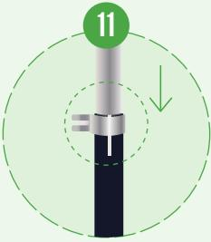
On the side opposite to the holding button, line up the Collar Clamp with the main stem recess groove and push into place
