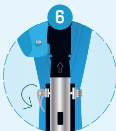
Close handle lock mechanism by flipping down the lever
