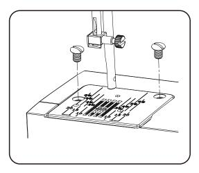
With a brush, clean out dust and lint clogging on the feed dog teeth. Reset the needle plate.
