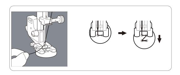
Position your fabric and button under the presser foot. Lower presser foot. Turn the handwheel to make sure needle clears both left and right openings of button. Adjust width if required. Sew 10 stitches across.
