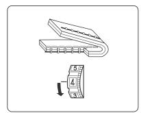
Tighten the needle thread tension by moving the dial to a higher number.
