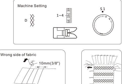
With the stitch length "4", sew straight stitching; lines 3/8 apart across the area to be smocked.Knot the threads along one edge, pull the bobbin threads and distribute the gathers evenly. Secure the thread at the other end.Sew the decorative stitch between the gathering stitches.Pull out the gathering stitches.
