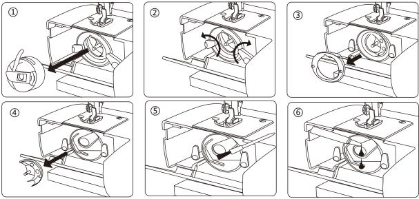
Raise the needle to its highest position and open the shuttle cover.
