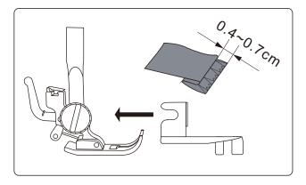
Raise the presser foot and place the fabric under the foot so that the soft fold rests against the wall of hem guide.
