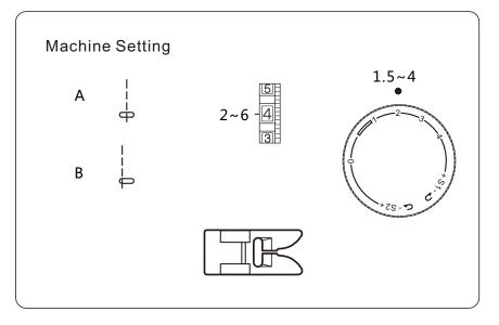
Raise the presser foot and position the fabric next to a stitching guide line on the needle plate. Lower the needle into the fabric. Lower the presser foot and smooth the thread towards the back. Depress the foot control.
