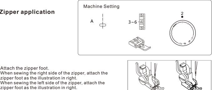
Helpful hint: During zipper inserting, ensure that the needle do not touch the zipper. Otherwise it will cause needle break or even injury.
