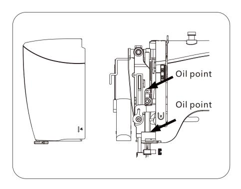
Apply a few drops of fine quality sewing machine oil to the point indicated by the arrows in the figures. For machine in constant use, oil two or three times a year.
