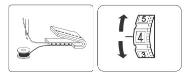
The top thread and the bobbin thread should interlock in the center of two layers of fabric in straight seams. Set the desired number of the thread tension dial at setting mark.
