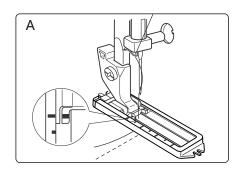
A. Select 🛛 , draw both thread to the left under the foot. Insert the garment under the foot.
