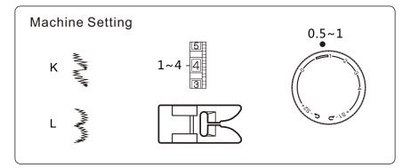
Sew a row of stitches and adjust the thread tension so the upper thread should appear on the reverse side of the fabric.
