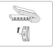
Loosen the needle thread tension by moving the dial to a lower number.
