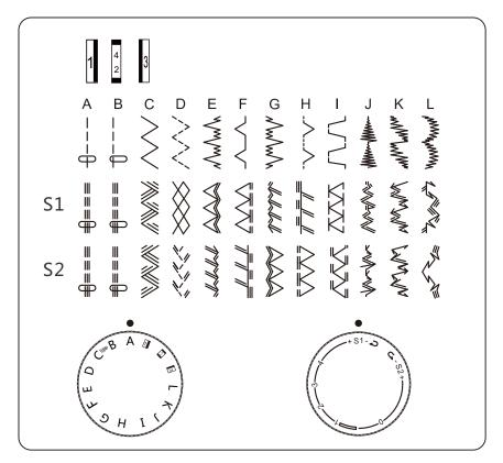
Raise the needle above the fabric and select the desired pattern at the setting mark by turning the pattern selector dial.
