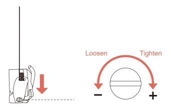
If the tension is correct, the thread will unwind by about 1-2 inches. If the tension is too tight, it will not unwind.
