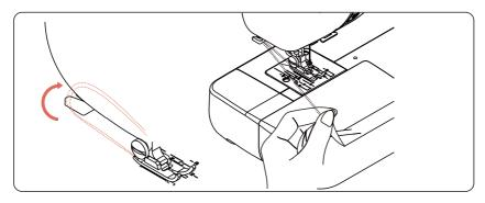
Pull the fabric and threads about 6inch (15cm) backward, then cut threads with the thread cutter from back to front.
