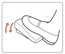
Place the fabric under the presser foot,put down the presser foot. When you have finished, remove your foot from the foot controller, then the sewing machine will stop.
