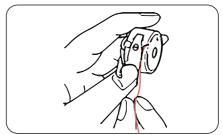
Note: The bobbin turns clockwise in the bobbin case.
