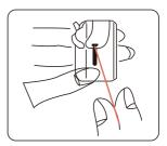
When you pull the thread, the bobbin should spin clockwise.
