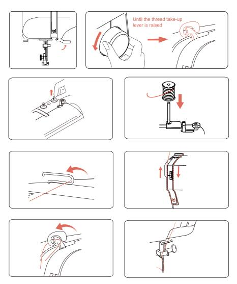
Note: Pass the thread through the eye of the needle from the front. For the convenience of threading, you can use scissors to cut off the excess thread.
