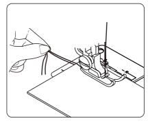
Pull the top thread and bobbin thread towards the back of the machine under the presser foot, until they are about 6inch (15cm) long.
