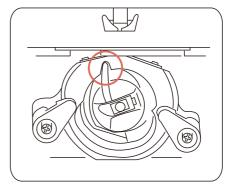
The pin on the case that should fit into the gap of the shuttle race.
