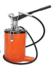
Manual grease dispensing system includes spring loaded pump, booster control handle, follower plate, and 9' hose. Simply pump the handle until it stays in the down position indicating the hose is pressurized.
