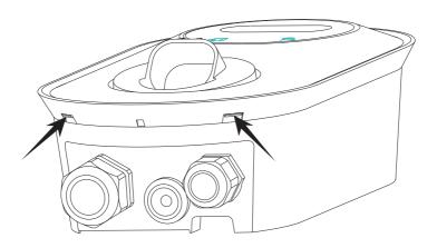
**2.** Loosen the six screws securing the second cover and carefully detach it from the base box.
