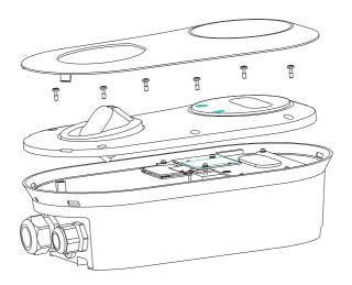
**3.** Remove the four screws per the diagram and gently lift the screen panel.
