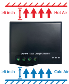
Figure 2.1 Installation and Heat Dissipation
