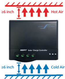
Figure 2.1 Installation and Heat Dissipation
