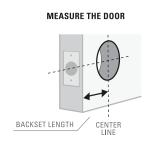
Measure distance between center of crossbore and edge of door.
