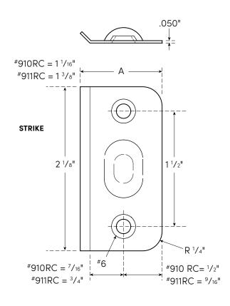
Fasteners Included: 4 ea. #6 x <sup>3</sup>/<sub>4</sub>" Flat Head Sheet Metal Screws
