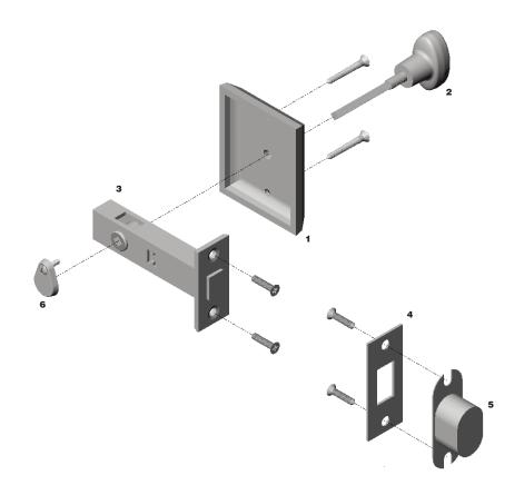
Note: Cut Shank on Turn Piece so that it goes halfway through the Mortise Bolt. This will allow a space for the emergency release key to operate the Mortise Bolt.
