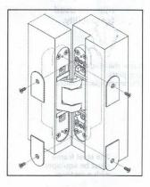
Screw the small cover plates using the enclosed tapping screws onto frame and door part.
