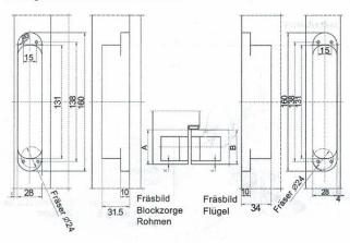
Calculation of milling dimensions: A = Frame rebate depth up to sealing level, B = Door leaf thickness or first door rebate: A - B + 4 = Dimension X The result must be a dimension between 4 mm and max. 7 mm. (Steel frame: X = 5 mm)
