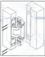
Fasten hinge frame part depending on the frame type. If required, please loose slightly the upper clamping screws for the height adjustment.
