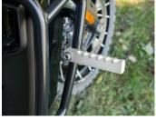
With a 3/16" hex wrench, remove half of the clamping collar, and loosely place each peg in the preferred location on the protection bar on your motorcycle. Reinstall the other half of the clamping collar, and evenly space the gaps on each side of the collar, with the screws only finger tight.
