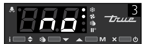
Image 3: If "no" appears on screen, the controller is unlocked.
