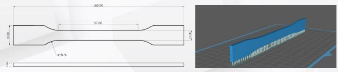
Testing prints setting: 0.05mm/layer, default setting, bottom layer exposure 30s, layer exposure 3s, print by Elegoo Mars 3.
