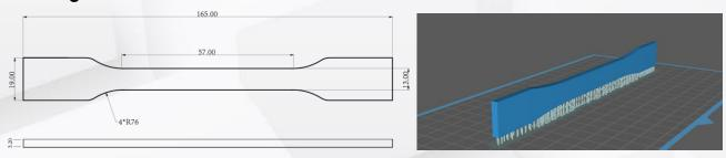
Testing prints setting: 0.05mm/layer, default setting, bottom layer exposure 30s, layer exposure 3s, print by Elegoo Mars 3.
