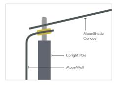
Orient MoonWall to match the side where you are installing it. Lift MoonShade canopy off of one upright support pole. Place the appropriate adjustable grommet tab of MoonWall onto the support pole post, and replace MoonShade canopy grommet over MoonWall grommet.
