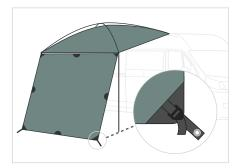
Once both bottom corners of MoonWall are staked, tighten MoonWall's grommet slides until MoonWall is taut. You may need to adjust the position of the stakes to achieve the best position and tautness for MoonWall.
