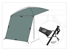
Grab one unused stake. Insert the pointed end of the stake into one of the bottom cordage loops of the MoonWall. Choose the desired angle for MoonWall to hang, anywhere between vertical and 45° outward from MoonShade. Secure MoonWall in place by driving the stake into the ground at a 45° angle, until the stake's hook is lodged in the ground. Repeat with an unused stake on the second bottom grommet.
