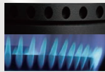
Oversized burner ports
