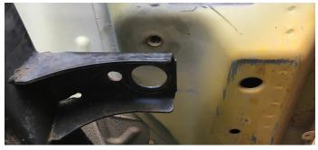
**STEP 3.** Using either a plasma cutter or a grinder with a cut off wheel, remove the factory body mount. Grind the frame smooth around the body mount until it is bright shiny metal. This will ensure a good surface to weld to.
